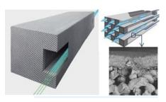
Crystar® FT dead-end technology are highly permeable silicon carbide membranes for liquid filtration. They are certified for swimming pool and drinking water according to standards NSF61/50. Silicon carbide is characterized by high chemical stability and abrasion resistance, as well as an excellent trade-off between retention efficiency and permeate flux.
