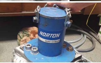
To guarantee a state-of-the-art refractory installation result, we provide high-quality installation equipment such as forks or pneumatic rammers (Bosch-type vibrator, bottom vibrator or Klein-type sidewall vibrator).
