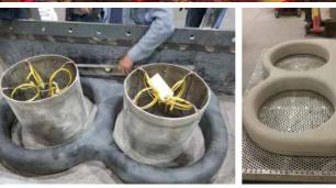
Customized precast ceramic loops for inductors ensure competitive downtime and ease of installation in inductors by providing additional safety and lifetime in operations.
