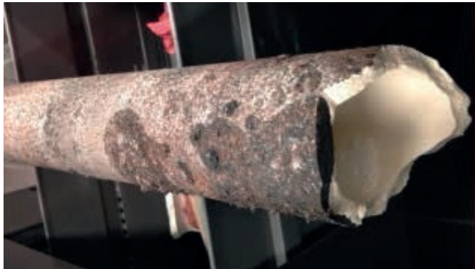
Mullite rollers after six months
