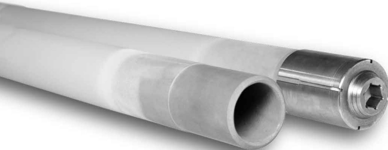
SiC rollers after 12 months - Superficial contamination with no penetration into the body
