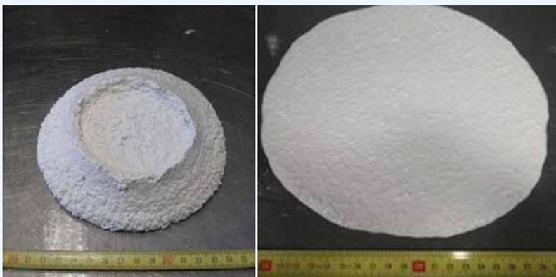
Comparison of flow properties of standard castable mix (left) and **Norflow®** (right), both samples having the same weight, grain-size distribution and water content. **Norflow®** spreads more, thus the self-flowing property is more developed.
