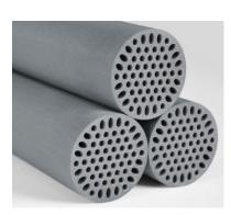
**Crystar® FT** are highly permeable and pure silicon carbide crossflow membranes for liquid filtration. They are certified for food contact according to the European regulation 1935-2004 and deemed acceptable for food and beverage contact by the FDA. Crystar® FT membranes are characterized by high chemical and thermal stabilities, superior thermomechanical and abrasion resistances and an excellent trade-off between retention efficiency and permeate flux.
