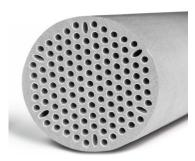
Crystar® FT are highly permeable and pure silicon carbide crossflow membranes for liquid filtration. They are certified for food contact according to the European regulation 1935-2004 and deemed acceptable for food and beverage contact by the FDA. Crystar® FT membranes are characterized by high chemical and thermal stabilities, superior thermomechanical and abrasion resistances and an excellent trade-off between retention efficiency and permeate flux.
