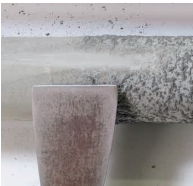
SiC rollers after 12 months – Superficial contamination with no penetration into the body
