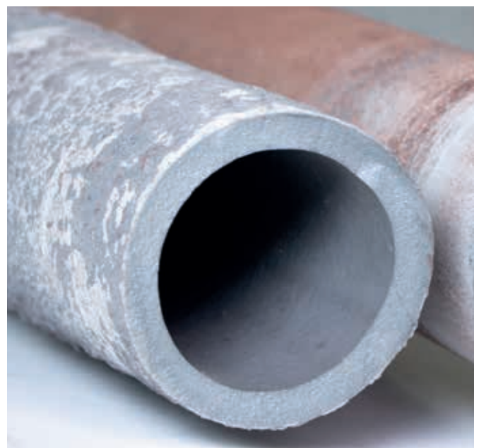
SiC rollers after 12 months – Superficial contamination with no penetration into the body
