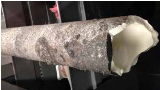
Mullite rollers after six months
