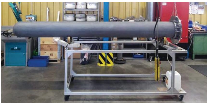
Fig. 3. SiC radiant tube (courtesy of Elster GmbH)
