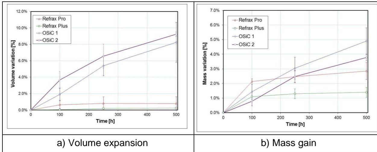
Figure 3: Volume expansion and mass gain induced by steam oxidation
