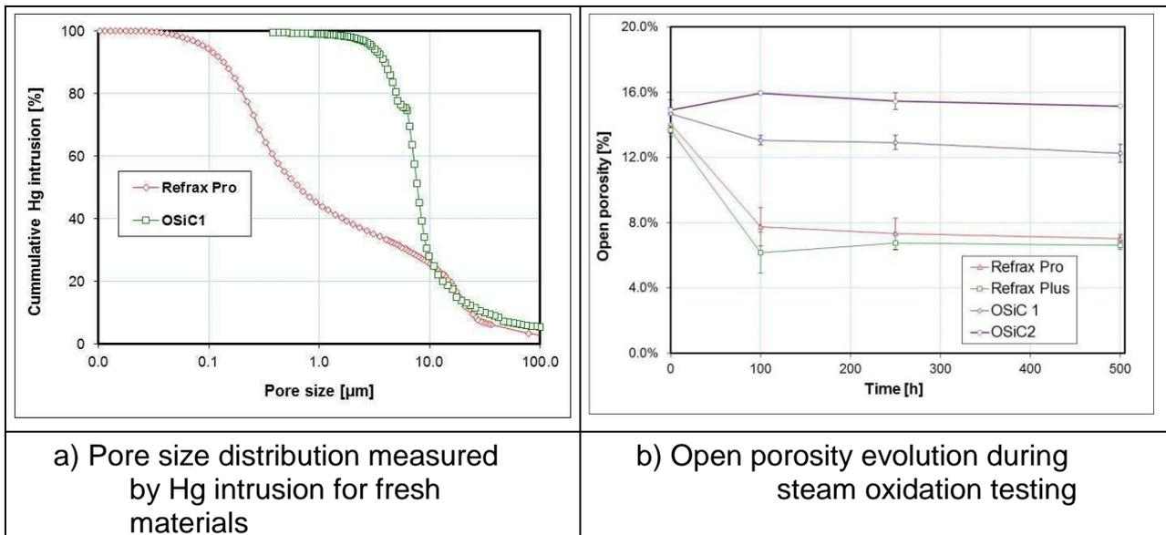
Figure 4: Comparison between OSiC and NSiC microstructure characteristics (initial pore size distribution and open porosity evolution during steam oxidation)
