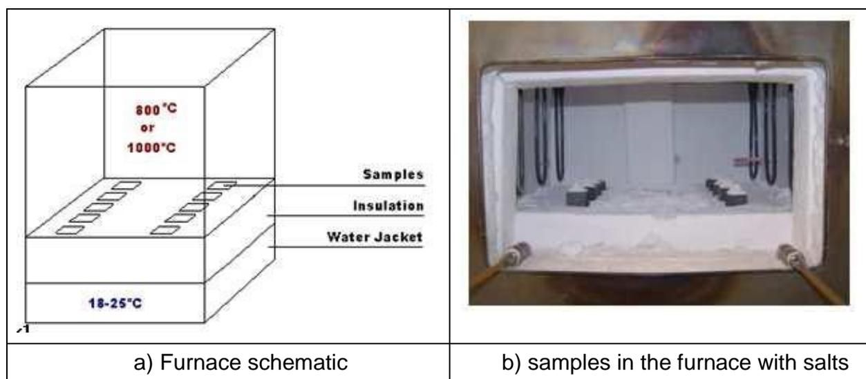
Figure 2: Salts corrosion/oxidation test configuration
