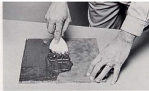
2. Apply from 1/16 inch to 1/8 inch depth (FOR STEEL SURFACE)
